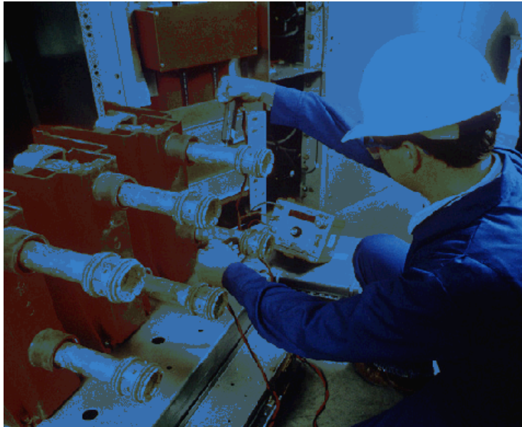
Figure 6-3—Contact resistance testing
